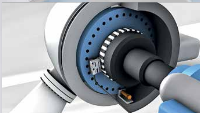
rotational speed monitoring on wind power generators
