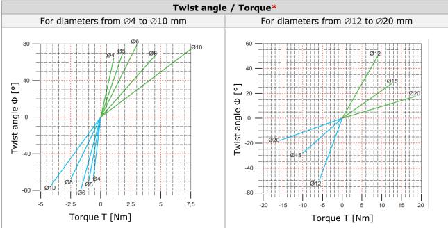
\* The data refer to flexible shafts with a total length of 1000 mm.
