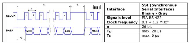
\* The maximum frequency is guaranteed with a cable length up to 2 m.
