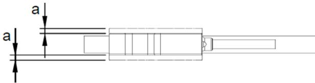
$$a = 3_{\text{MAX}} \text{ IMS1-}_{-}\text{C}$$
