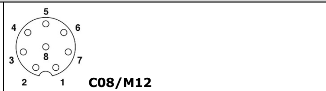
Schematic drawing: Pin diagram connector (socket) M12, 8-pin, A-coded, view socket side
